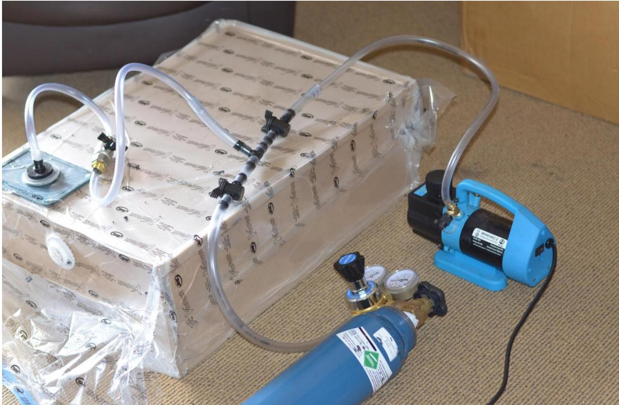
Figure 3: Complete assembly showing argon bottle, PVC tubing, T-connector and valves to switch between evacuation and back-filling, rotary vacuum pump, vacuum bag and the inner wood vacuum chamber. The vacuum chamber contains the plastic bag with a herbarium box (fig. 6) and is fully evacuated in this photograph.
