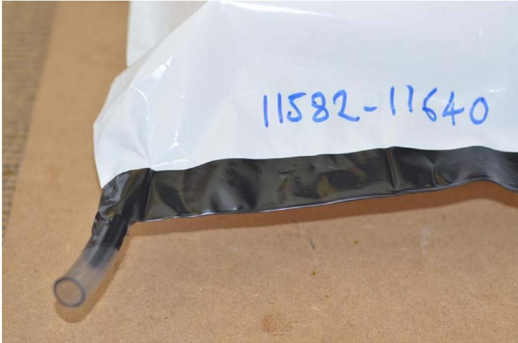
Figure 6: The herbarium box is enclosed in a gas-impermeable plastic bag which is sealed with PVC tape, with a tube inserted at one end to allow evacuation and argon back-fill. On removal from chamber the tube is pulled out and remaining gap sealed.
