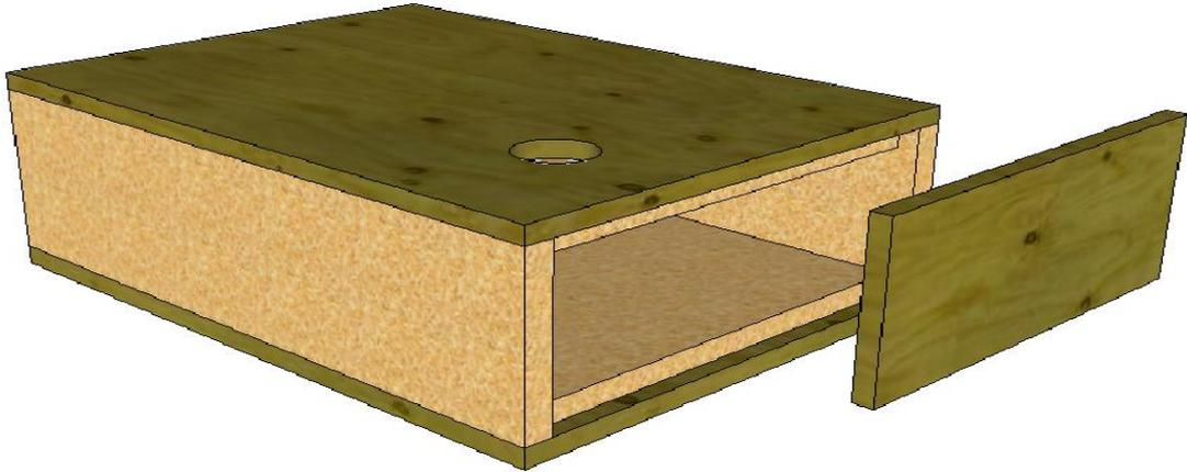
**Figure 1:** Construction of the wooden vacuum chamber. Note the arrangement of the double-layer wall of the box and the recessed end-lid, thus ensuring the force of the vacuum is distributed across the length of the walls.
