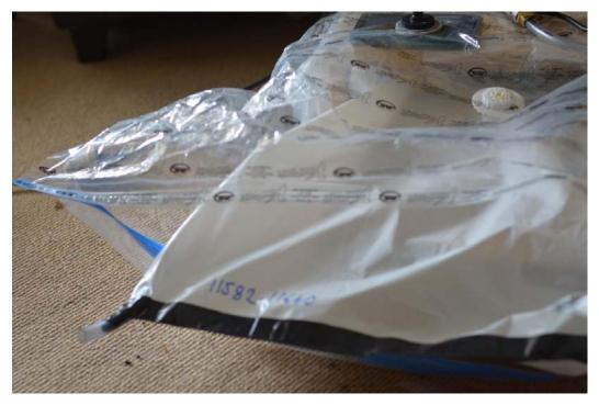
Figure 7: The herbarium box and enclosing bag with protruding tube is inserted into the vacuum chamber inside the vacuum bag which is then sealed.
