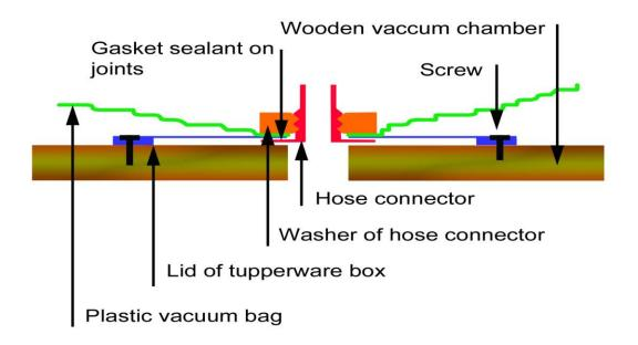
**Figure 2:** Details of the vacuum-tight joint between an external hose-connector, the plastic vacuum bag, and the internal wooden chamber.
