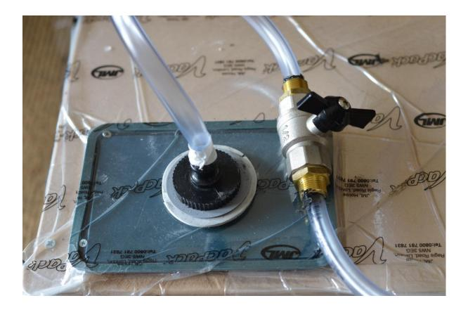
Figure 4: Connection to vacuum bag and chamber, showing vacuum-tight ball-valve.
